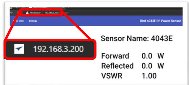
Now plug in your sensors with the provided power supply and connect the LAN port to your computer. Then open a web browser and enter the sensors default IP address (192.168.3.200) in the address bar and press Enter. You should now see the sensors built-in webpage.
