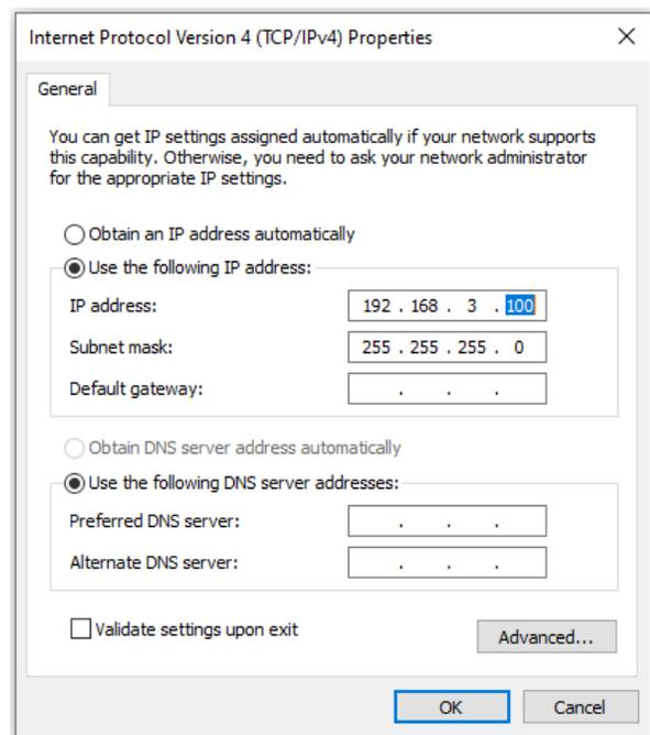
Enter the IP address and set the first three octets to 192.168.3. The fourth octet can be set to any number between 1 and 255, except for 200 which is reserved for the sensor. For this example, 100 was used. Then
