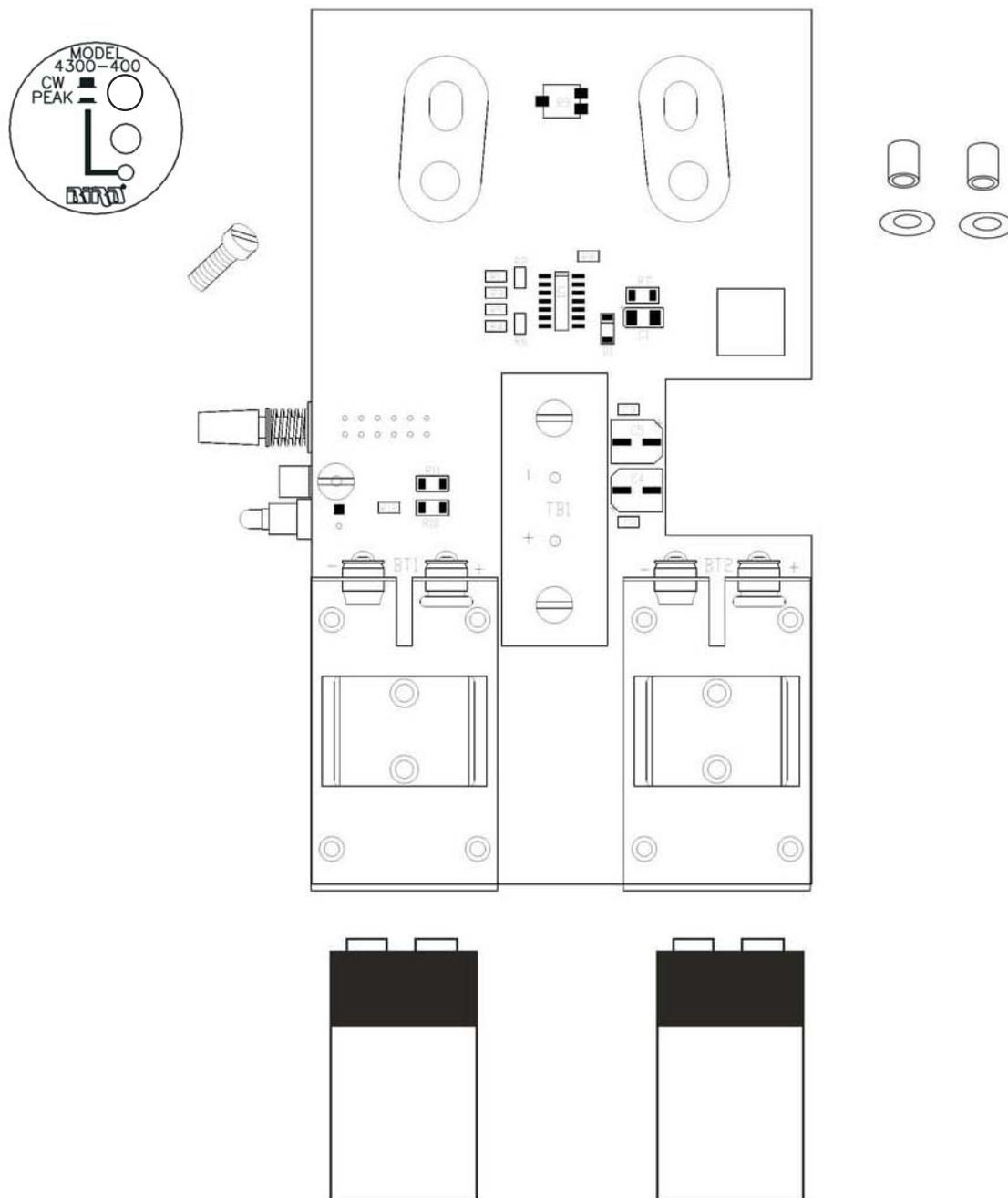
Figure 3 Model 43P Open Showing 4300-400 Kit Installed
